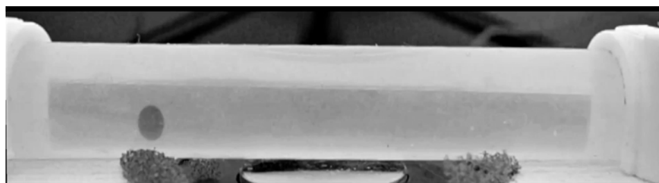
Figure 8. Side view of a fragment of the experimental setup for positioning the ferrogel bead in a magnetic field. The diameter of the bead is about 2.4 mm. See explanation in the text.
