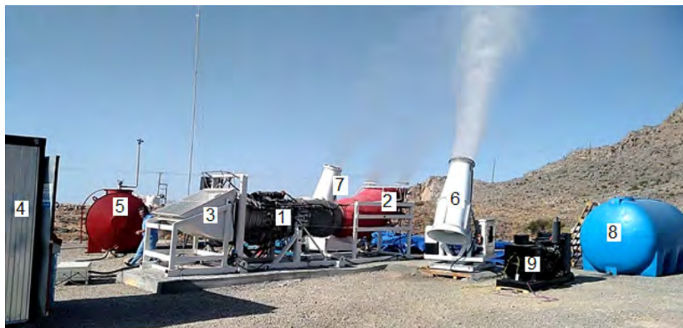
Figure 6. Experimental complex in operation: (1) aircraft engine D-30; (2) nozzle for directing the jet up; (3) engine air receiver; (4) engine start and control cabinet; (5) jet fuel tank; (6) Fog Cannon JY-60; (7) Fog Cannon WP-60; (8) tank for hygroscopic substances solutions; (9) diesel generator 3 \times 380 50 kW to feed the Fog Cannon JY-60.
